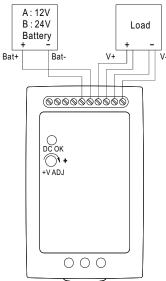
Fig 1.1 Suggested system connection
